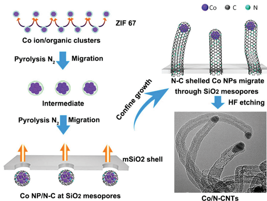
Fig. 4 Formation mechanism of Co/N-CNTs.
